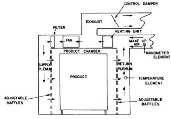
Figure 1—Example of a dry heat sterilizer for convection batch process
