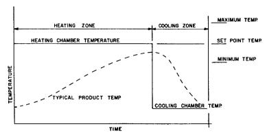
Figure 5—Example of a continuous cycle
