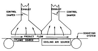
Figure 3—Example of a flame sterilizer for continuous conduction process
