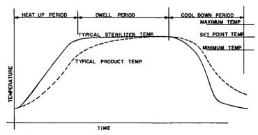
Figure 4-Example of a batch process
