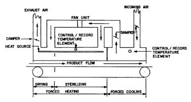
Figure 2—Example of a dry heat sterilizer for convection continuous process
