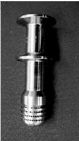
FIGURE 8 If a filter housing is fitted with nozzles in the top dome area, a spray-type device of short length and capable of being drilled for a wide variety of flow and pressure requirements is used to direct streams to the multiple nozzles, as when cleaning larger vessels.
