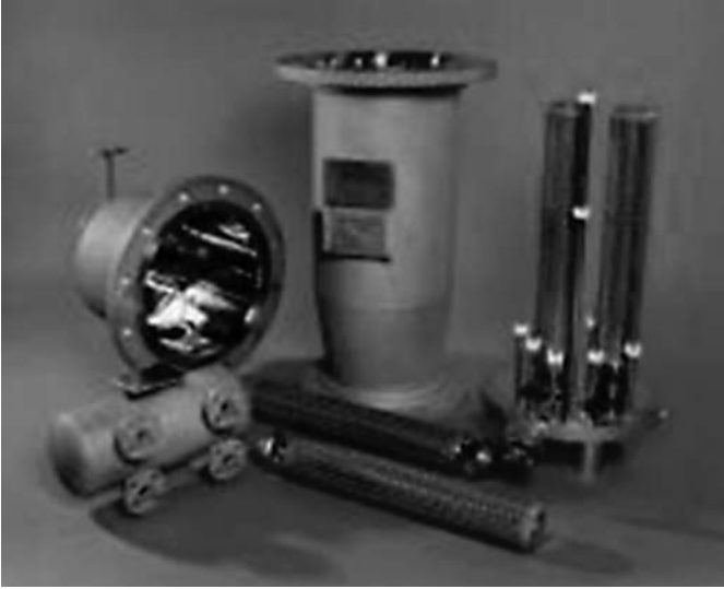
FIGURE 12 Disassembled stainless filters in baghouse. Source: Courtesy of Fisher-Klosterman, Inc.
