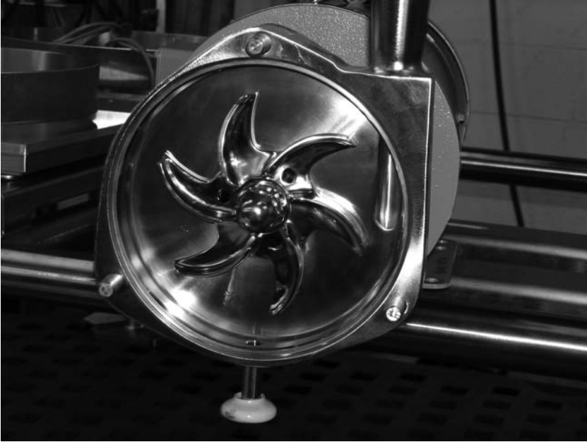
FIGURE 13 Hygienic impeller retaining nut.
