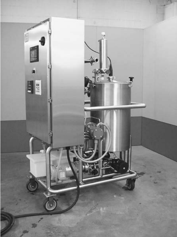
FIGURE 17 This mini-CIP skid is used for demonstrating fully automated CIP to an aseptic process course and a cleaning validation course. Source: Courtesy of the Parenteral Drug Association (PDA)-Training and Research Institute (TRI).
