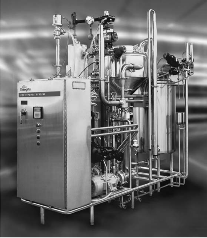
FIGURE 13 A single-use eductor-assisted CIP skid with one water tank. Note tangential inlet on air separation tank above eductor.
