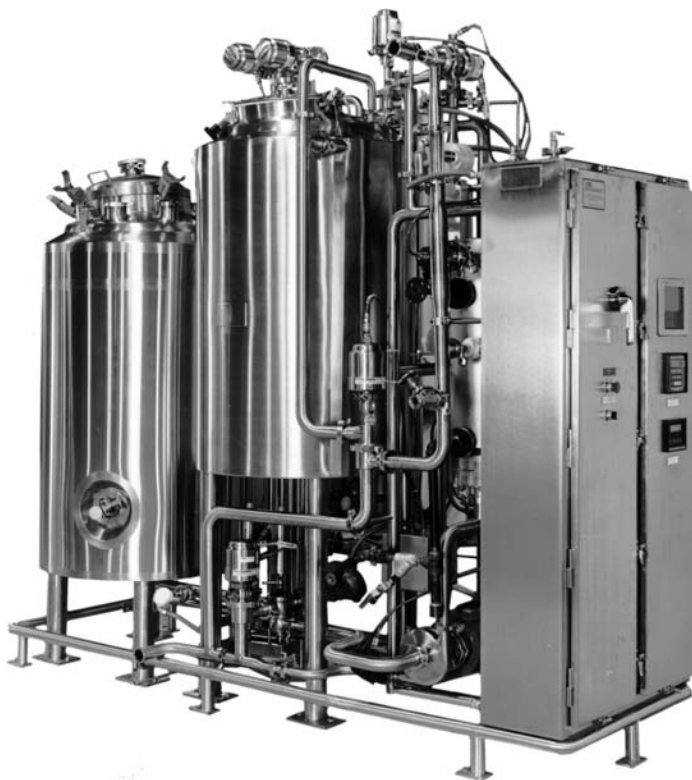
FIGURE 11 This clean-in-place skid combined the use of a CIP recycle tank on the return side of the circuit with the ability to operate as a single-pass CIP skid. The large water surge tank was required to accommodate a low flow rate water-for-injection loop.
