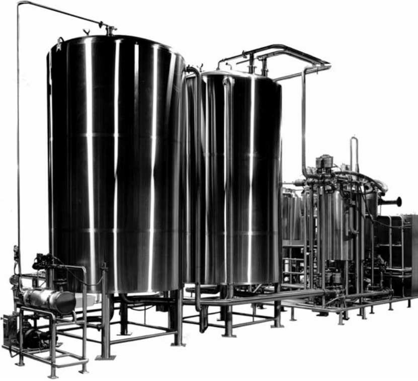
FIGURE 15 This large CIP skid included two single-use total-recycle systems operating at up to 200 gal/min supported by large pure water and neutralization tanks.
