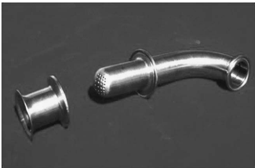
FIGURE 6 This specific "bubble spray" and installation sleeve were designed for installation in the sidewall of a screw conveyor. The bubble projects only slightly through the installation ferrule and, if necessary, can be made flush.
