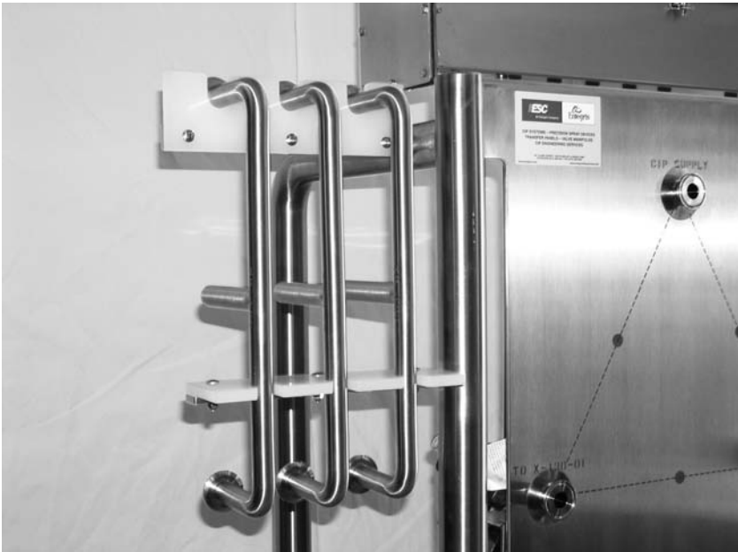
FIGURE 7 U-bends with magnet assemblies.
