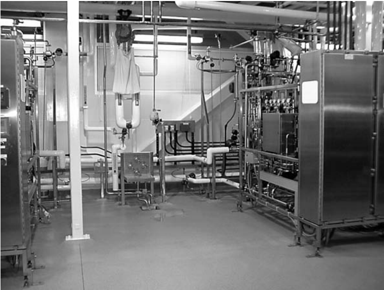
FIGURE 12 This photograph shows two small bioreactors depicted schematically in Figure 11 connected to a common transfer panel for harvest/CIP flow selection.
