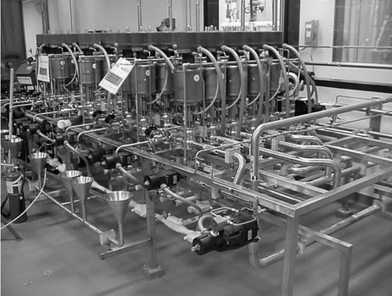
FIGURE 7 A second lower-level mixproof valve manifold controlled flow from the ten hold tanks to the four columns. The design provided for CIP of all piping to and from a selected hold tank in combination with the vessel under fully automated control.
