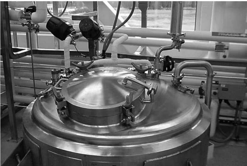
FIGURE 2 This view of a media prep vessel illustrates the high manway collar and also the rupture disc, vent filter, and level indicator nozzles that create clean-in-place spray coverage problems.
