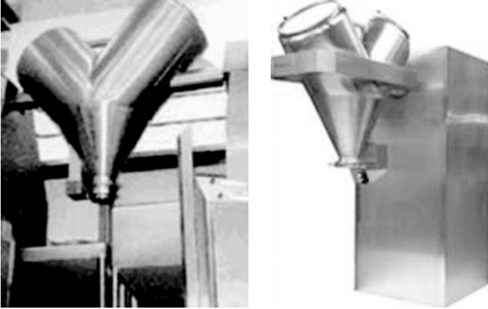
FIGURE 17 Sanitary V benders. Source: Courtesy of Pharmatech Ltd.
