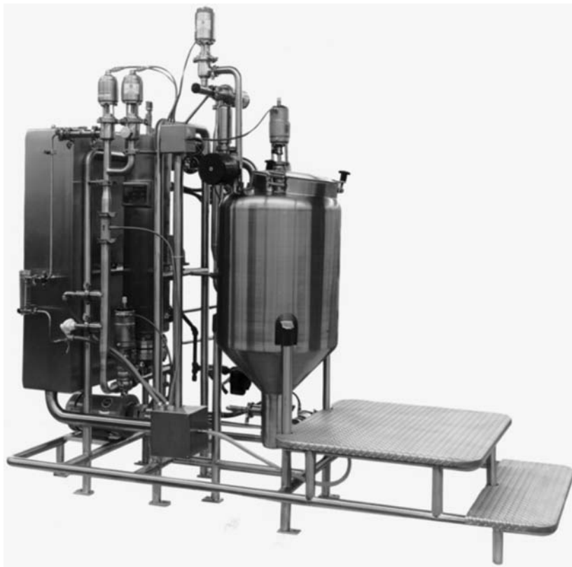
FIGURE 16 This CIP skid is a drug mixing system that can clean four mixing tanks, and all associated piping to three downstream processes.
