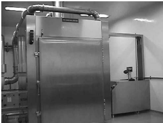
FIGURE 36.2.2 Bin-washing station (side view).
