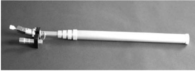
FIGURE 43.1 Remote swabbing and microbiological sampling tool.
