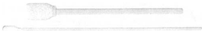
Figure 10.1. Typical swabs used for swabbing for chemical residues (courtesy of the Texwipe Company LLC).
